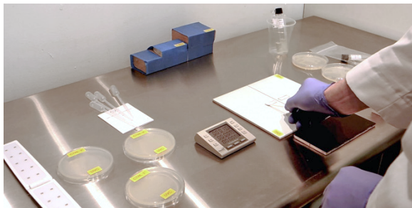
Figure 5: Ceramic tile being dosed with E. Coli and then being treated with the UVC wand.
